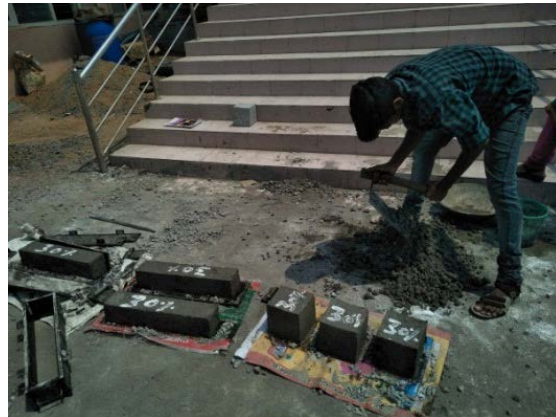
Fig.6: Concrete placed in moulds
